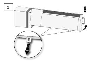
Position the base station slightly tilted onto the DIN rail and latch it in.
