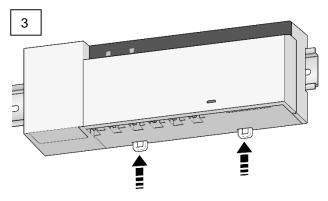
Fix the Base Station securely with the locking mechanism on the DIN rail.
