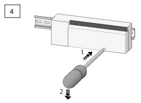
Remove the cover with a screwdriver.
